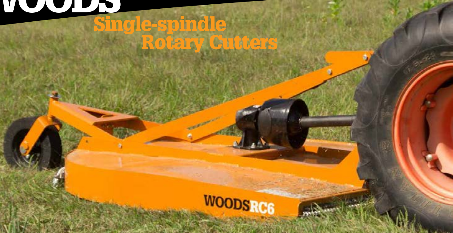
RC6 shown with optional chain shielding
