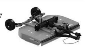
WARNING: CHAIN SAFETY SHIELDING STANDARD EQUIPMENT. Chain safety shielding must be used for all non-agricultural uses and in areas where the possibility of thrown objects could be hazardous to persons or property. The maximum transport speed for towed and semi-mounted machines is 20 mph (32 KM/H). Regardless of the maximum speed capability of the towing tractor, do not exceed the implement's maximum transport speed.
